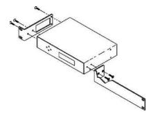
Attach a long and short rack ear to each side at the front of the unit, using five of the 8-32 x 1/4" screws.
