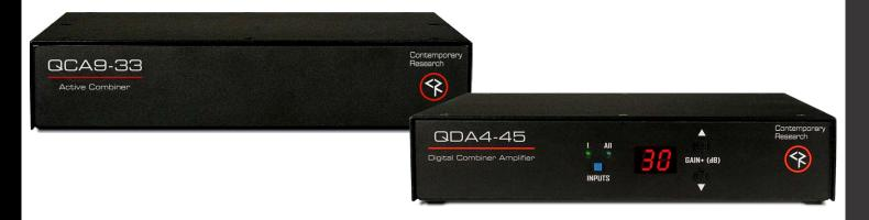
The Contemporary Research Q series of RF distribution components represents a fresh solution for RF channel combining and amplification. The **QCA9-33** starts by actively combining at low 30 dB levels, with no loss and little noise, then feeding the **QDA4-45** for a final 45-50 dB level with only a small net gain in noise.
