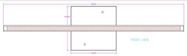
The LA-B18 is a low voltage, remote controllable, visual signaling device. The 17.5 by 0.5 inch RGB LED optical element has programmable color and intensity which may be stored as a preset. The preset can be recalled by Ethernet or RS-232 serial command or by contact closure.
